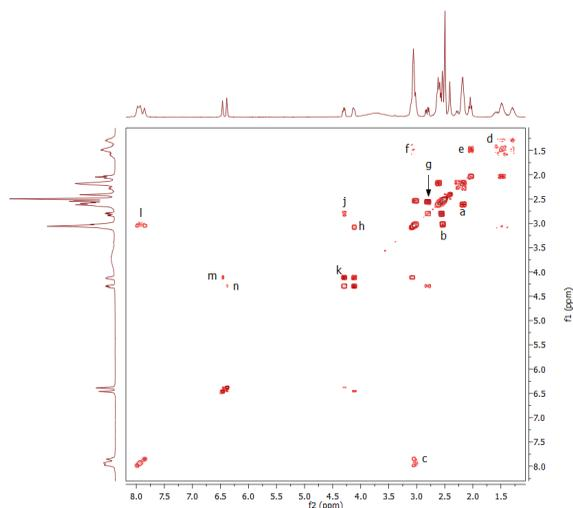
**Fig. 3.**  $^1\text{H}$ - $^1\text{H}$  COSY spectrum of  $G_0$ -Biot in  $\text{dmsd}_6$ . The relevant off-diagonal peaks are labeled in right-lower part for dendrimer and left-upper part for biotin
