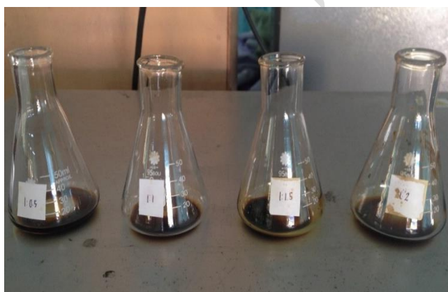
Fig. 1. Synthesized C-Nanodots from Kamias at varying amount of monoethanolamine
